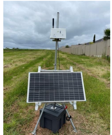
Solar-powered dust monitor.
