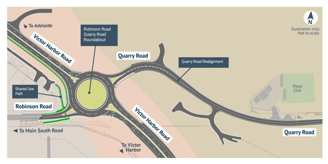
As part of the Victor Harbor Road Duplication project, the intersection at Robinson Road and Quarry Road will become a roundabout. Quarry Road will be realigned to meet Robinson Road. The roundabout will provide continuous traffic flow and safety improvements.
